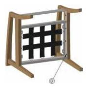
**D:** Using a #2 Philips screwdriver remove the end frames from the metal seat frames. On double or triple seat configurations you will need to do the same with the center arms.
