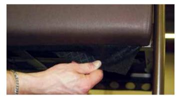
A: Remove the upholstered seat cushion by pulling away the Velcro® tabs at the front and rear of the cushion.
